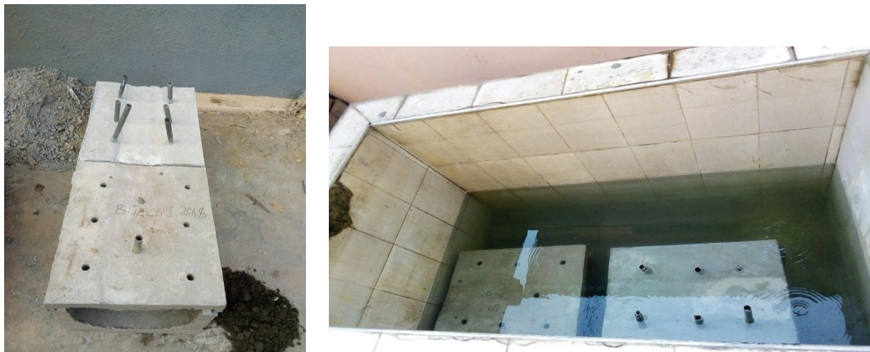
Figure 3. Test samples and curing stage
