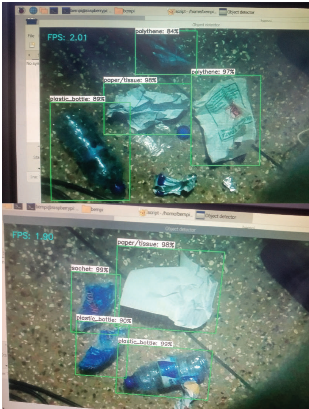
Figure 6: Litter Detection via Raspberry Pi Webcam
