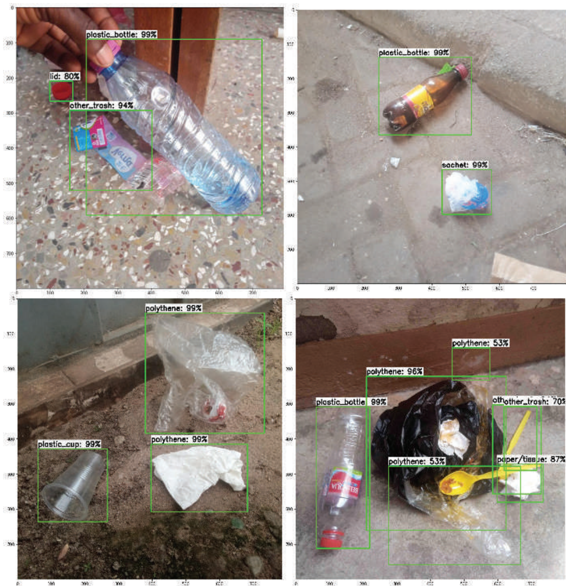
Figure 5: Litter Detector Model Performance Evaluation on Test Data
